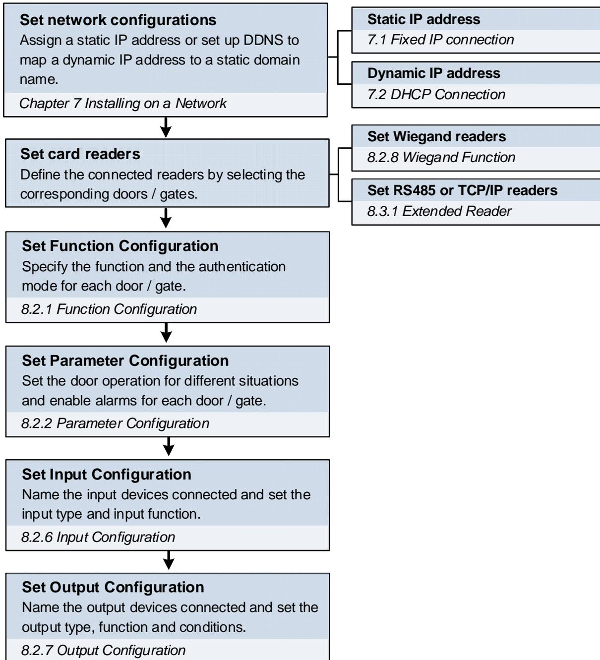
**Note:** The Wiegand Function and Output Settings pages are not available for GV-AS1010 / 1110 and GV-EV48. For GV-EV48, the Input Setting page is also not available.
