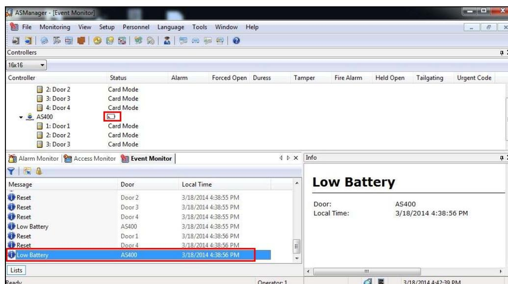
**Note:** Make sure the plastic insulation film under the battery is removed when using GV-AS100 / 2110 / 2120 / 4110 / 8110 for the first time. The low battery messages and icons will appear if the plastic film is not removed.
