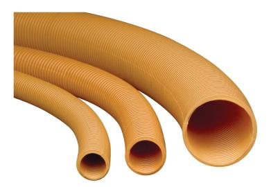
Ideal for providing a main chase from the main distribution panel to a secondary hub in the attic or basement, Resi-Gard non-metallic flexible raceway is available in  $\mbox{\em 4"}$  to 2" diameter sizes with factoryinstalled pull tape in sizes 1" to 2". The raceway is hand bendable, lightweight and easily cut to length to reduce scrap. Bright orange color clearly signifies a low-voltage installation.
