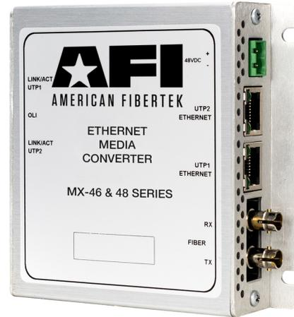
The American Fibertek 46-PoE+ Series transmits and receives (2) copper 10/100/1000BASE-T Ethernet signals at the RJ45 ports and (1) optical 100 Base-FX over 1 or 2 multimode fibers. The system is comprised of two units forming a point-to-point communications link.
