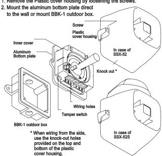
3. Plastic cover housing can be hooked-up as per drawing.
