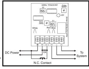
Note: The application is for use with DC power <u>only</u>. It <u>WILL NOT</u> work with AC powering and/or tripping the CVM-60.
