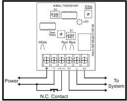
at which time, the relay immediately drops out. If the N.C. contact is re-closed before the end of the time delay, the relay never activates, the timer resets and awaits the next contact closure.
