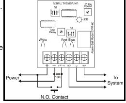
potentiometer, the relay activates and remains active until the N.O. contact is opened, at which time, the relay immediately drops out. If the N.O. contact is re-opened before the end of the time delay, the relay never activates, the timer resets and awaits the next contact closure.
