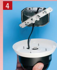
4 With camera mounted, install the mounting plate to the box by placing it on the bracket and turning clockwise to lock. Install set screw.
