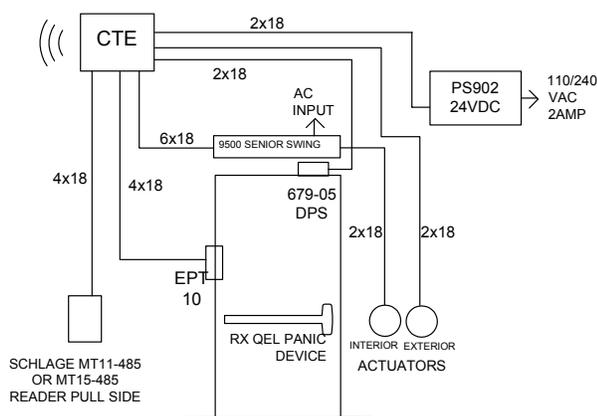
**Operation:** Presenting a valid credential to Schlage MTBXX will cause QEL panic device to retract for authorized entrance and enable exterior actuator. Free non-alarmed egress at all times. Interior actuator always active to retract QEL panic and open door.
