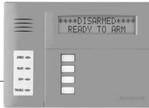
The 6160CR is an addressable remote keypad intended for use in commercial fire applications with ADEMCO's control platforms. The keys are continuously backlit for convenience and easy visibility. The LCD display is backlit only when a key is depressed\*, or when the system is in alarm or trouble condition.
