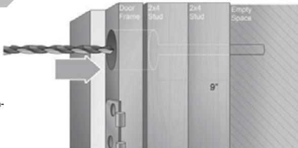
A 1/4" hole must now be drilled in the center of the cavity through the door jamb. This is so the antenna can be inserted through the door jamb frame and the supporting studs.
