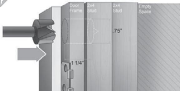
Use a 3/4" drill bit to drill into the door jamb to a 1 1/4" depth.
