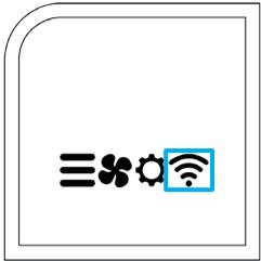
This icon opens the Smart Hub network connection menu. In this menu, you can choose to connect or disconnect from your Smart Hub. Select “SET” to establish a new Smart Hub connection. Select “OFF” to temporarily disable the connection. Lastly, select “ON” to reconnect to your Smart Hub. For more information about connecting to a Smart Hub, please view KONOzw’s Smart Hub Setup Guide.
