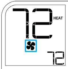
The active fan status is shown by the icon below the ambient room temperature. If it is off, your fan is not running. If it is on, your fan is running. Please note that your fan will run depending on your selected fan mode (either AUTO or ON).
