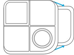
Securely fasten KONOzw onto its base. Once it has clicked into place, return power to your heating and cooling system.
