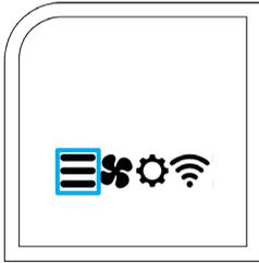
This icon opens the system mode menu. In this menu, you can set your HVAC system to OFF, HEAT, or COOL. Your thermostat will automatically detect which modes are available when you install your thermostat, so you may not see all three options depending on your system type.
