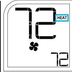
The selected system mode (HEAT, COOL or OFF) is shown to the right of the ambient room temperature.
