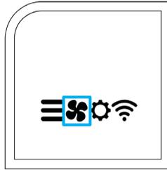
This icon opens the fan mode menu. In this menu, you can set your fan to AUTO, or ON. AUTO will run your fan when your system is actively heating or cooling. ON will run your fan continuously. If you set a filter life value in the installation settings, you'll be able to check the remaining life of your filter in the fan settings menu.
