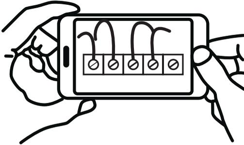
**Step 1.5:** Use the included wire labels to mark which wire is connected to each terminal in your old thermostat.
