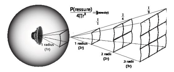
The other side of this equation is that you would have to increase the power to the loudspeaker by 6dB- or four times the power to "even up". Remember that the loudspeaker taps are in 3dB increments either twice-or half the power of the adjacent tap.
