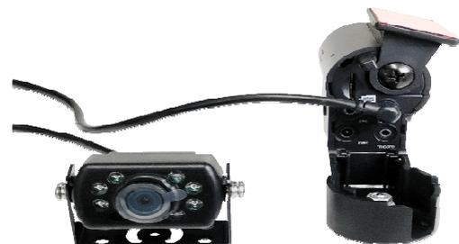
Connect the (optional) EX6-OMIR camera with video cable provide. Connect to VIDEO Input port on the VDR-600
