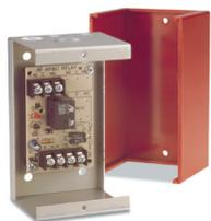
Each relay position contains a red LED which indicates the relay coil is energized. Relays may be "snapped apart" from a standard 4 module assembly and used independently. These Devices are Ideal for applications where local contacts are required for system status, remote contacts for control of electrical loads and general purpose switching. They are suitable for use with HVAC, Temperature Control, Fire Alarm, Security, Energy Management and Lighting Control Systems.
