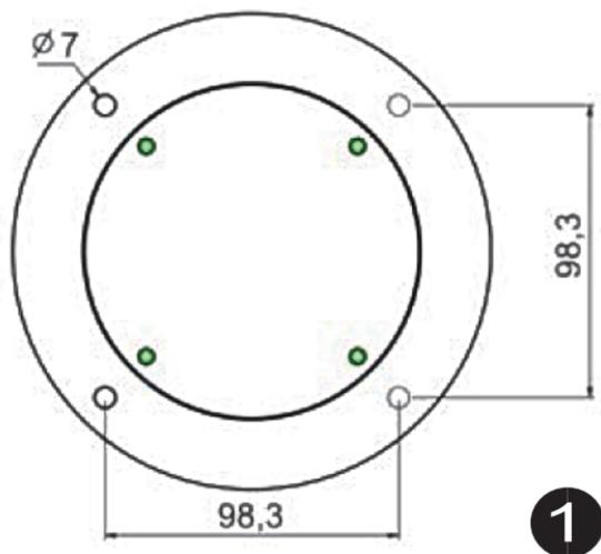
2. Drill holes on the ceiling for securing the pendant head. Secure the pendant head by hammering anchors into the ceiling and then fasten screws through it.
