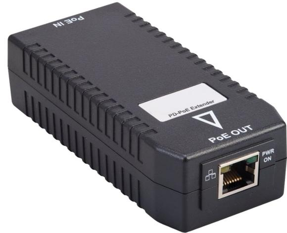
The **POE130-XT** is a single-port Power over Ethernet (PoE) Gigabit extender that is designed to meet the demanding data rate and power requirements of IP cameras with high-quality streaming video capabilities. A single PoE extender can repeat Ethernet up to 200 meters. When cascading three extenders with a PD9601G midspan injector, Ethernet and PoE can extend up to 400 meters (1640.42 feet) to an IEEE802.3af device.
