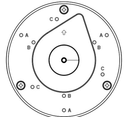
**5** Pass the camera's Ethernet cable through the center hole of the box and the rubber seal.
