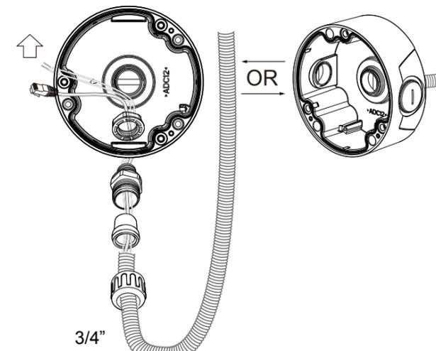
**7** Make sure the rubber seal is properly installed to the center hole. The outer rim of the seal must be through and cover the edge of the hole.
