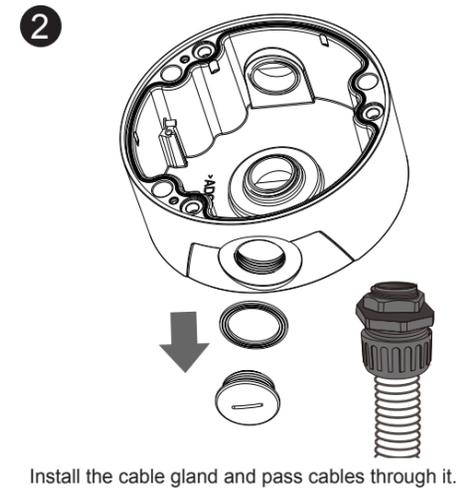
Install the cable gland and pass cables through it.
