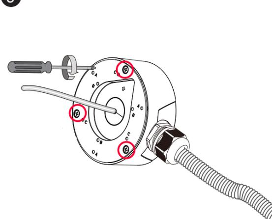
**10** Install the camera using the corresponding mounting holes.
