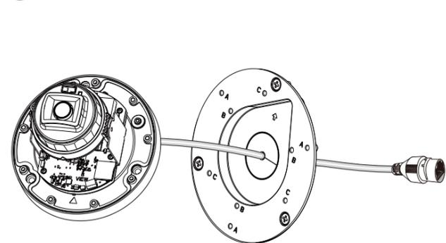
**6** Install the waterproof components of the cable gland to your Ethernet cable following the QIG of your camera. The cable gland will be placed within the protection of the box.
