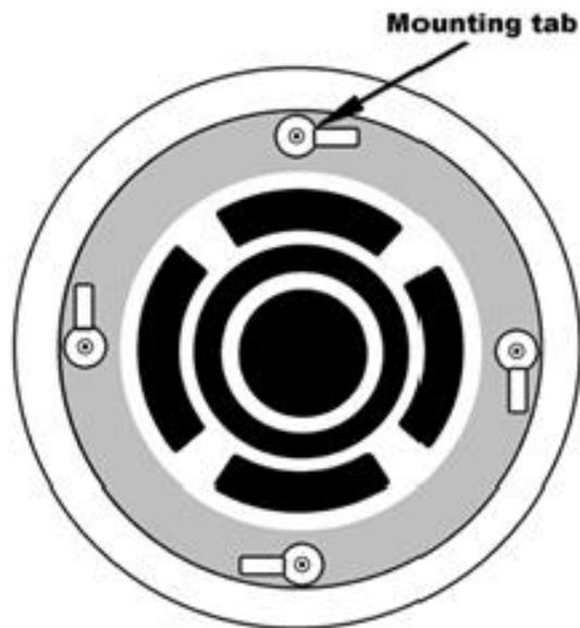
Be sure to position the four Mounting Tabs on your OWI speaker inward then insert the four (4) screws (supplied) from the front of the speaker into the screw opening.
