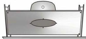
3. After hole is cut in the ceiling, connect the wires and install the speaker by tightening the screws of the four clamps.
