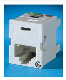
Clarity 6a, 6 & 5e TracJacks, ETL verified to TIA Category 6a, 6 & 5e component specification. Front-loading and front removable. New universal T568A/B wiring label and tapered wiring towers simplify termination. Center tuned to Clarity patch cords for optimum performance.
