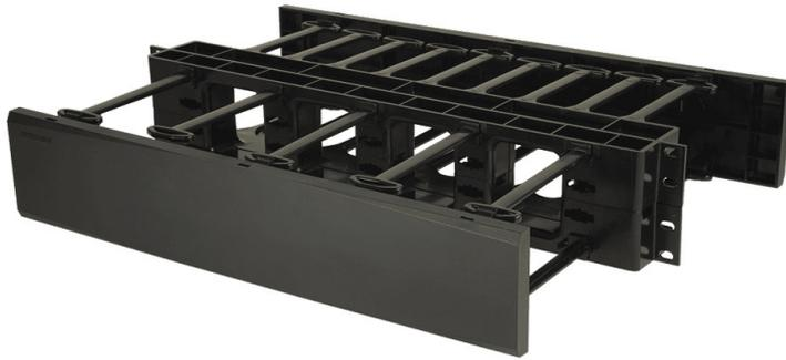
Legrand® horizontal cable managers are available in 1RU, 2RU, 3RU & 4RU sizes. Fingers begin 3/4" from the face of rack to provide bend limitation for cables, protecting cables, equipment and network performance. Included hinged cover mounts with six heavy duty clips allow them to be opened one handed without becoming "unhinged". Manufactured from UL94V-0 rated plastic. Available in Black and White.
