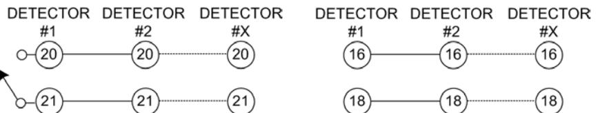
Common test/reset. 30 detectors max. (Use normally open test/reset switch)
