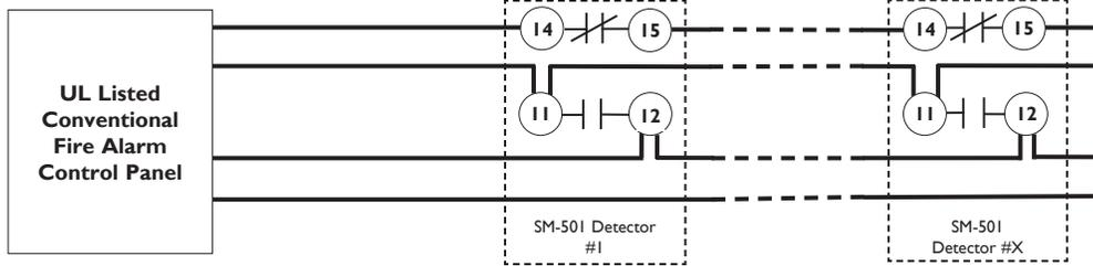
**SAMPLE CONTROL PANEL WIRING - STYLE "B" / CLASS "B" IDC** (Supervised - A fault condition will not inhibit an alarm response)
