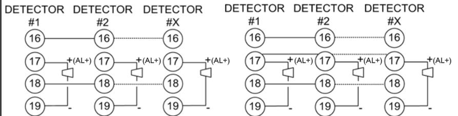
All alarm relays operate with single alarm. Individual horn/strobe units operate on any single alarmed detector only. 30 detectors max.
