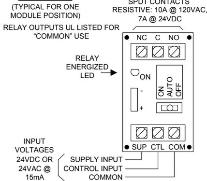
**NOTE:** SUPPLY (SUP) AND CONTROL (CTL) INPUT MUST BE OF SAME VOLTAGE TYPE AND POLARITY
