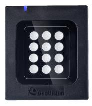
The GV-RK1352 is a card reader with keypad, designed to recognize PIN codes, identification cards or both. Featured with the Wiegand and RS-485 outputs, the unit can be connected to any standard access control panel. GV-RK1352 comes with a weather sealed and IP66 compliant housing for outdoor use.
