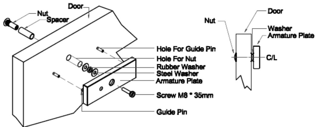
Typical Installation of the electromagnetic lock:
