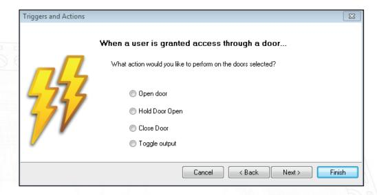
You can directly control a door lock by selecting an action on this screen. The open door function unlocks the door for the 'Door open time' and it then relocks.
