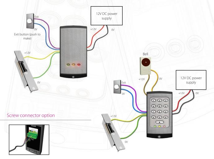
Screw connection versions of the 75 series may be mounted in conjunction with an electrical backbox. This allows the pre-wiring of installations where the wiring is in conduit.
