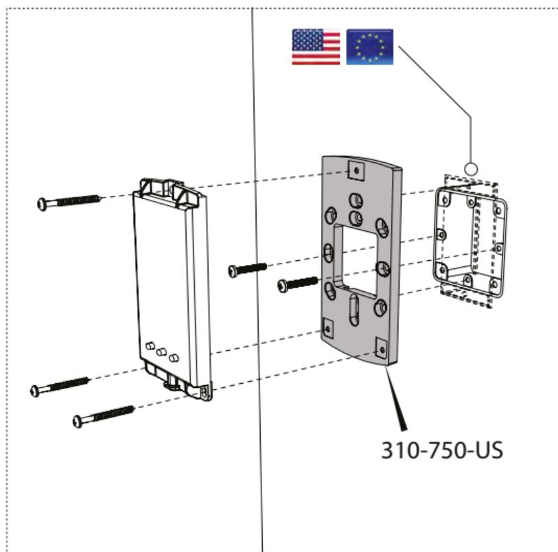
If a 75 series backbox adaptor kit (310-750-US) is fitted, the mountings on a backbox can also be used.
