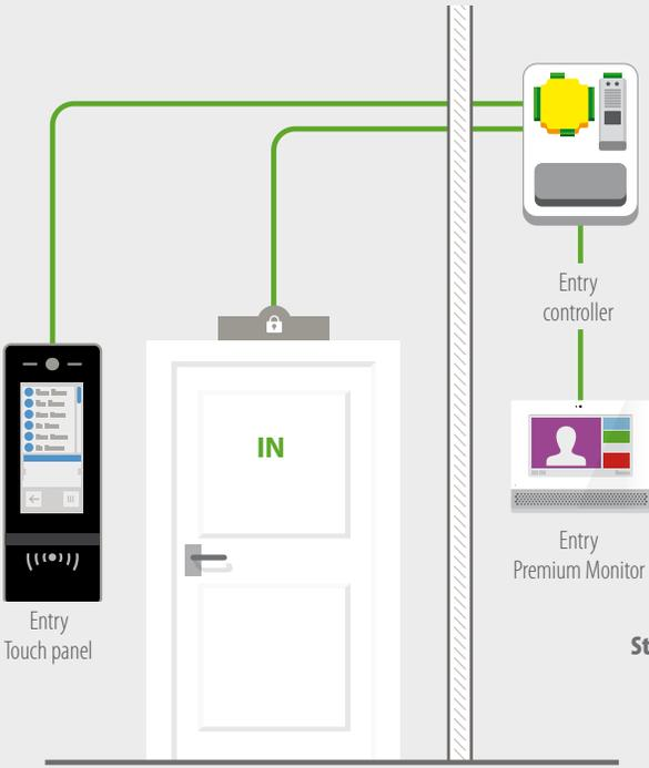
**Standalone Entry system does not require connection to a network or server**
