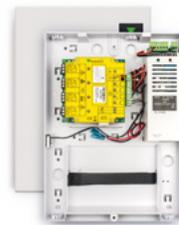
Net2 I/O board with 2A PSU in plastic cabinet
