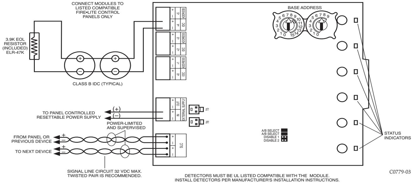
1. To use a common power supply between multiple MMF-302-6 modules, connect a long power supply jumper from T5 or T6 to T5 or T6 on the adjacent MMF-302-6 module.
