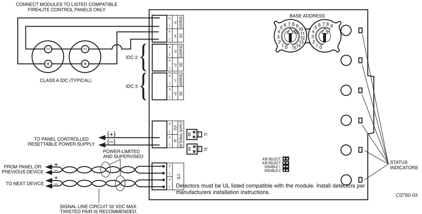
1. To select Class A, remove the two shunts from the "A/B select" positions.
