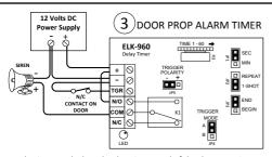
Delay is started when the door is opened. If the door remains opened after the time delay has expired the relay will turn on and remain on until the door is closed. If the door is closed before the time delay expires the ELK-960 is reset awaiting another input from the door contact.
