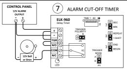
Useful for adding a cut-off timer to a control panel that does not have one. It can also be used to shorten the cut-off timer for a control with no adjustable timer.
