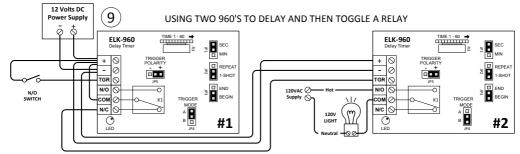
Used for delaying a trigger then toggling a relay on/off. ELK-960 #1 starts a time delay when the N/O switch is closed. When 960 #1's time delay expires, 960 #2 is triggered turning it's relay on for the time delay setting, then turning the relay off. (toggle) To sumarize: fire trigger on #1, waits, turns on #2's relay, waits, then turns relay off.
