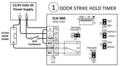
Used to extend the release time of an access control device or to manually activate a door **strike** release device. The trigger is activated by a contact closure or a N/O pushbutton and the door strike remains activated (door open) after the button is released for the delay time set up in the ELK-960.
