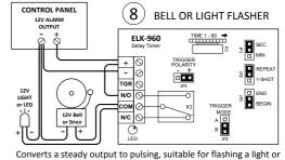
pulsing an audible device. Note: Alarm output must be capable of supplying enough current to drive the bell and light.
