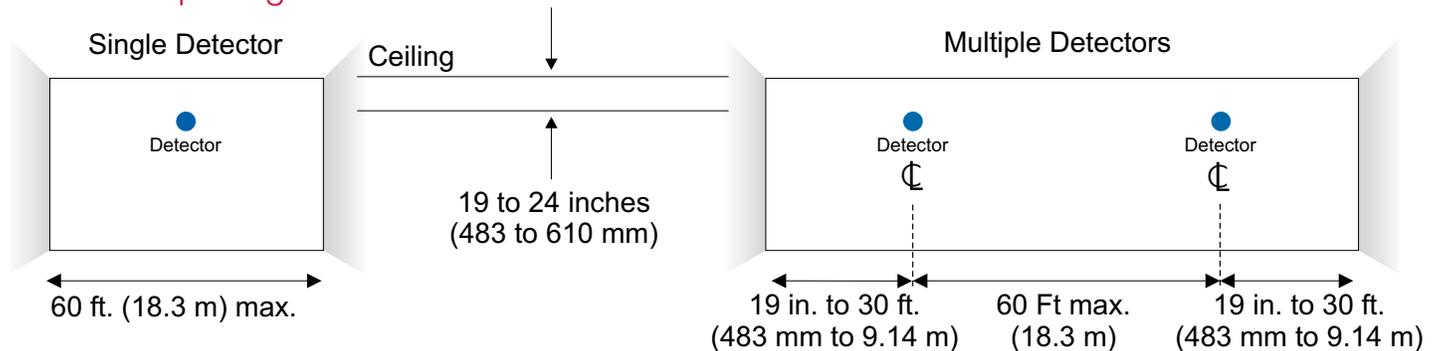
Detector positioning shown here is recommended for protected areas with flat ceilings. Spacing may vary for areas with high or sloped ceilings. In such cases, verify operation with smoke tests.
