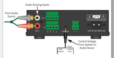
The A120 is audio-sensing so anytime an audio signal hits the A120 inputs, the amp will instantly turn ON. The amp will turn itself OFF after 15 minutes when no audio signal is present. The 12VDC Trigger input will turn the A120 ON when 12-24VDC is applied and turn the amp OFF when the voltage is removed.
