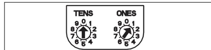
Figure 2.4: Address switches
