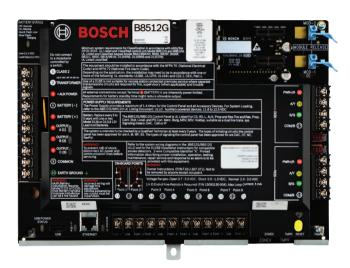
The B9512G Control Panel and the B8512G Control Panel are the new premier commercial control panels from Bosch. B8512G control panels integrate intrusion, fire, and access control providing one simple user interface for all systems. With the ability to adapt to large and small applications, the B8512G provides up to 99 individually identified points that can be split into 8 areas.
