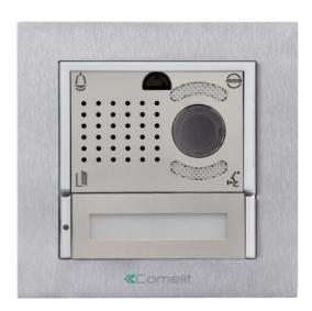
Single-family video door entry external unit for ViP system with Ikall Metal entrance panel. The kit comprises: 1 flush-mounted box Art. 3110/1, 1 silver coloured frame Art. 3311/1S, 1 module with 1 button art. 33411M and 1 colour audio/video unit Art. 4682HKE. The external unit is coded with ViP address 101 and the button on module Art. 33411M sends the call to ViP address 1. Compatible with H.264 video format.
