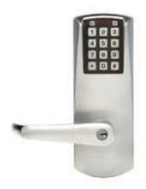
PowerPlex is a self-powered, electronic PIN push button lock that uses patented super-capacitor technology in place of batteries or external power sources to power the door lock, making it a cost-effective access control solution for stand-alone applications.
