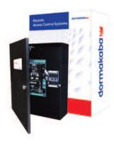
The Keyscan CA4500M is a network appliance-based access control unit that gives you unmatched flexibility for new installations or revitalizing aged or failing access control systems. The CA4500M is a package that includes 1 CA4500B ACU board, 1-OCB8 relay board, 1-DPS-15 power supply, and 1-black metal enclosure with lock and tamper switch. This unit is special order hardware programmed for up to 90,000 credentials. It functions only with Aurora software.
