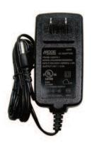
The PS1225 is a replacement 12VDC plug-in switching transformer for the SDACSKT (SDAC Kit). Plugs into standard 120 Vac outlet and provides up to 2.5 amps. Has 60" of 18 Gauge cable for mounting close to SDAC control. Has 2.1 mm barrel power connector. Center positive. For replacement of transformer provided in the SDACSKT. C/UL/US Listed Black Colour
