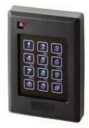
Farpointe Data single-gang mount Indala format proximity surface mount keypad reader. Dual reader and keypad. Wiegand output. Reads the Keyscan 125 kHz 36-bit Indala format. A HID PXK501 replacement reader. Black. 18" (457.2 mm) – 9 conductor shielded cable pigtail. Two-piece design with snap-on cover to hide mounting screws. Weight is 4 oz (113 g). Product Listings: UL294, FCC, IC. Warranty: Limited Lifetime.
