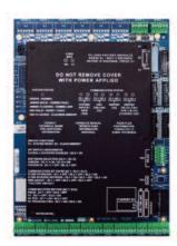
The Keyscan EC1500BM is an elevator floor access control panel only. It is available to replace non-functioning EC1500M access control panels.
