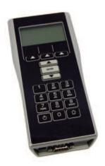
The E-Plex wireless site survey unit is used to determine the best and most efficient placements for new and existing E-Plex wireless systems.
