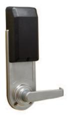
E-Plex wireless inside antenna kit with 4C batteries for use with E5600/E5700 Series locks. Converts E-Plex 5600 or 5700 hardware to operate with ZigBee wireless system integrating with Keyscan Aurora software. Includes antenna with back-plate and connecting cable; RF antenna is located on top of the E-Plex Lock. Enables optimum RF signal when a Gateway or Router is located on the opposite side of secure opening.
