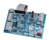
A new communication control module designed to use a CAN Bus communication network. The CIM provides optimized server to Access Control Unit (ACU) communication giving users an ACU to ACU network providing inter-panel communication for global functions. The CIM also includes enhanced device-based diagnostics and improved communication speeds.
