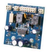
The Keyscan DPS-15 is a dual-linear DC power supply with two outputs for ACU-12VDC at 1.2 Amperes and AUX/RDR-12VDC at 1.2 Amperes.
