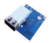
Networking a Keyscan access control unit is made easy by using the Keyscan NETCOM6P encrypted plug-on adaptor. Allows maximum system design options. NETCOM6P is designed to plug directly onto the CIM to establish network encrypted communication using CAN Bus communication network. You can also plug onto ACU board in other specific applications. Also available non-encrypted (see NETCOM2P).
