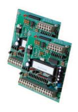
When circumstances dictate a long cable run between control panel and reader, exceeding 500 feet, rely on the Keyscan WIEEX2 wiegand extender. This interface converts the Wiegand signal to standard RS485 providing a communication range of up to 4000 feet between WIEEX2 receiver and WIEEX2 transmitter while using standard CAT5 cable between units.
