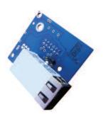
Networking a Keyscan access control unit is made easy by using the Keyscan NETCOM2P plug-on adaptor. Allows maximum system design options. NETCOM2P is designed to plug directly onto the CIM to establish network communication using CAN Bus communication network. You can also plug onto ACU board in other specific applications.
