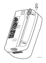
Remove tape from back housing and retrieve cover locking screw.
