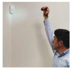
**Snap Walk Test:** Triggers walk test mode with the flick of a flashlight, reducing the number of trips to the sensor during installation.
