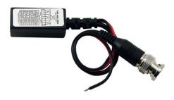
The CCTV Power-thru Balun provides the transmission of video signals and remote power via a single UTP (unshielded twisted pair) cable for more versatile cabling. The CCTV Power-thru Balun is used in pairs that allow you to eliminate more expensive coaxial cable, which include coupling signals from remote video cameras to display systems, video capture, security and surveillance monitoring applications.
