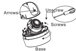
**Step 6** Aim the three through-holes on the camera base at the three swell plastic buttons in the ceiling, and use screws with a length of 30 mm to fix the base on the ceiling. Turn the main body clockwise for about 5 degrees to assembly it with the camera base, and fix the three screws, as shown in figure 3-6.
