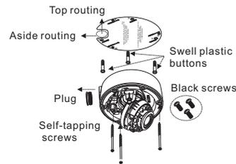
**Step 5** If camera base installation applied, press the arrows marked on the lining to remove the lining aside. Unscrew the three black screws and put them aside. Turn the camera base clockwise for 5 degrees and remove it, as shown in figure 3-5.
