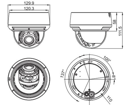
**Figure 2-5 Vandal dome Dimensions** Unit:mm
