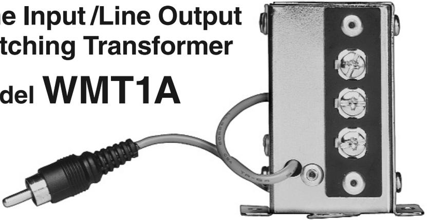
The **WMT1A** is a balanced and isolated impedance matching transformer. Typical uses are to provide a 600-ohm balanced input adapter for unbalanced AUX inputs. WMT1A can also be used to drive long, balanced, twisted pair cable. This improves noise rejection and the maximum run length. The WMT1A can adapt line-level signals down to levels suitable for MIC inputs. See the drawing below for setting the Operating Modes.
