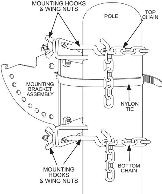
**IMPORTANT: HAND TIGHTEN ONLY. EXCESS TIGHTENING MAY CAUSE HOOK ENDS TO SPREAD.**
