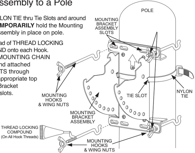
C) With Hooks fully extended, attach one end of MOUNTING CHAIN to one of the Top Mounting Hooks. Pull the Chain tight to Pole and then attach shortest link to corresponding Top Hook. (To keep chain from being jammed by the hook, place link on outside of the Hook.) Spin Wing Nuts down evenly, enough to keep the Assembly in place.
