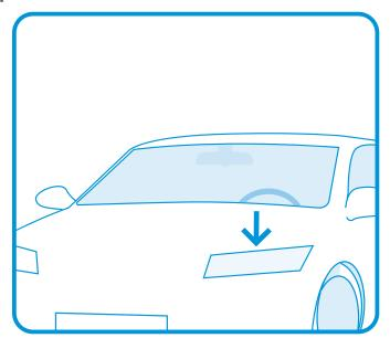
Determine the position of the UHF Exterior Tag on the headlight of the vehicle\*.
