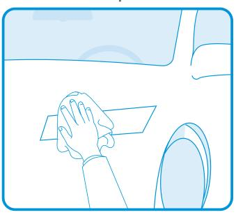
Clean the surface of the headlight. Make sure the headlight is free of oil and dirt. Degrease and dry the headlight with proper cleaning material.
