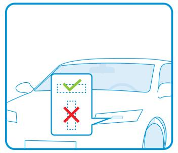
Remove the tag's protection layer before placing the tag on the headlight. The ideal temperature for mounting the tag is in between 10-15 degrees Celsius.
