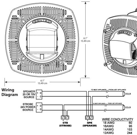
\* MAX. WIRE DISTANCE (IN FEET) = PANEL VOLTAGE - DEVICE MINIMUM VOLTAGE x WIRE CONDUCTIVITY (STROBE ONLY)
