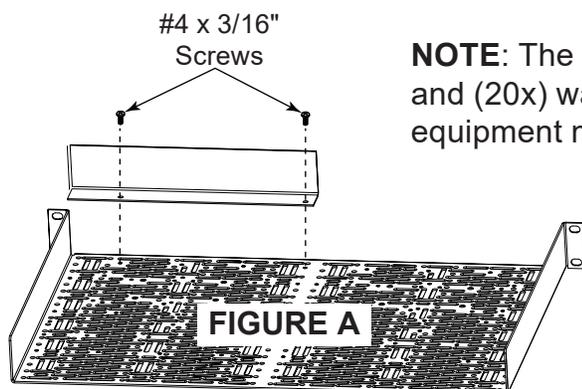
**NOTE:** The (4x) #6 3/16" screws, (16x) #4 3/16" screws, and (20x) washers are provided with shelves and kits for equipment mounting convenience.
