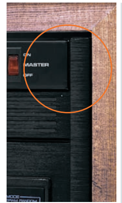
without trim strip installed
