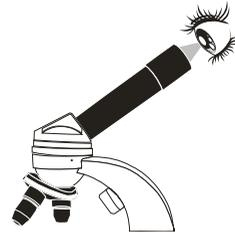
4. Select the appropriate rubber coupler size for the microscope eyepiece and insert it in the microscope adapter.
