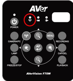
11. To disconnect the session, hit the **"Freeze/Stop"** button on the camera once. To reconnect, press and hold the "Wi-Fi" button until the Wi-Fi LED blinks. Connection to the either the AVer IFP or Dongle should take place after that.
