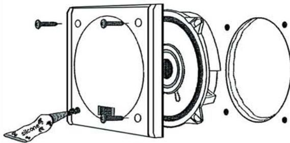
Both the M5CX and M4F weatherized speakers are held in place by (4) #8 stainless steel screws. Locate the speaker grill covers and put a small amount of silicone in screw holes. This will seal the screws. Using the Phillips screw driver, install the (4) #8 screws carefully aligning speaker in wall. (It is not necessary to seal the speaker grill cover - only the screw holes.)
