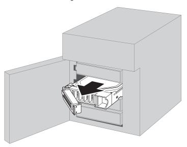
$oldsymbol{4}$  Insert the new drive into the empty slot with the lock mechanism remaining open.
