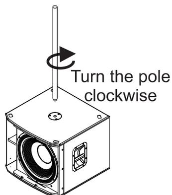
3. Turn the **M20 threaded pole** clockwise to secure the pole to the subwoofer.
