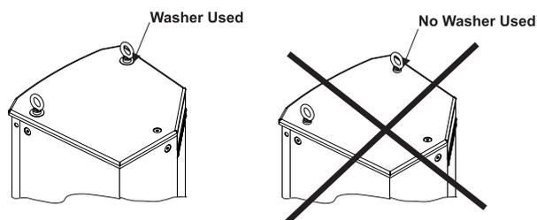
Figure 5.2: Eyebolt shown with and without washer
