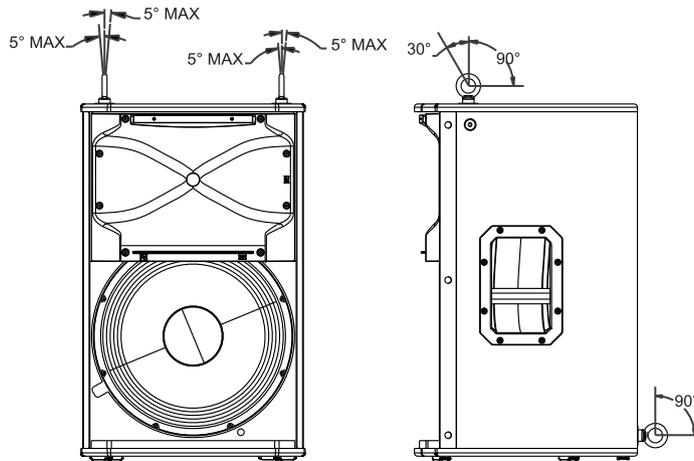
Figure 5.4: Maximum working load - vertical orientation
