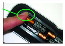
Now, replace the battery cover by inserting the hinged end in first, then snapping the cover back into place.
